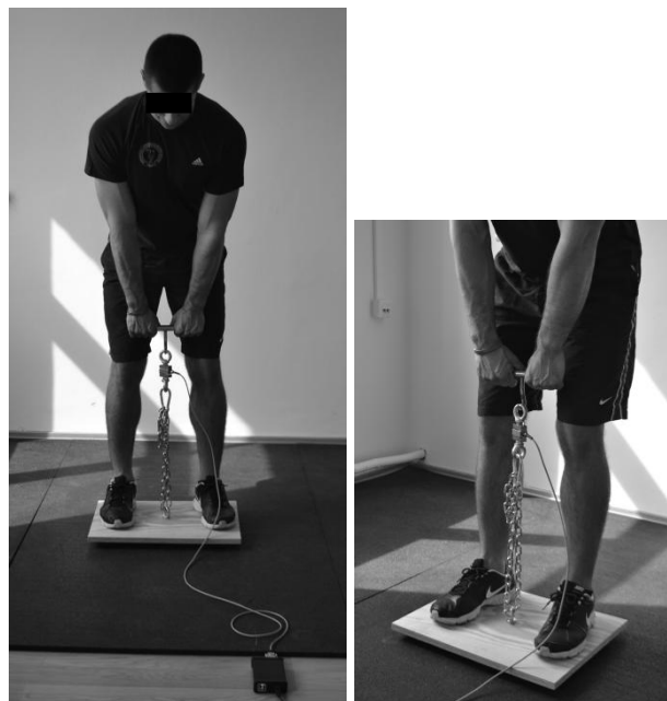
Figure 3 Assessment of maximal voluntary isometric strength using the FiTRO Back Dynamometer
