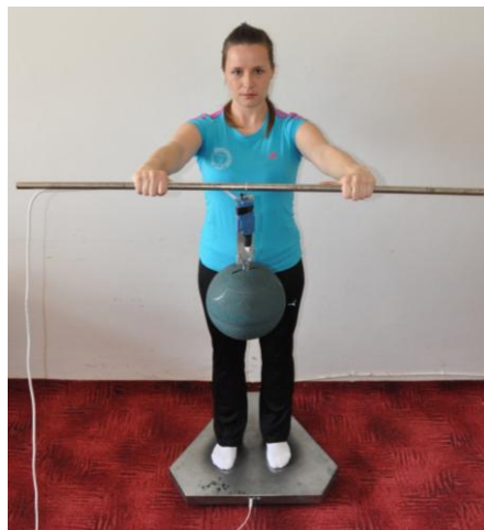
Figure 6 Load release balance test using the FiTRO Sway Check system completed with a special program for Load Release Balance Test
