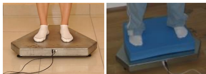
Figure 4 Standing on a force plate (a) and a foam surface placed on the force plate (b)
