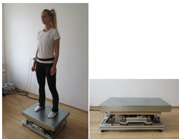
Figure 3 Tests of dynamic balance using the FiTRO Dynamic Posturography system
